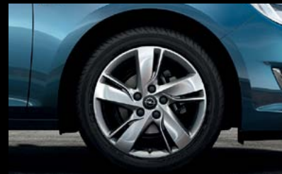
Lichtmetalen velg, 7 J x 17, 5 spaken, bandenmaat 215 (225)/50 R 17 (RTN). 3
