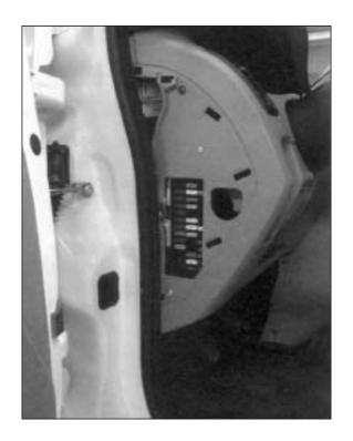
One fuse box on the left-hand side of the instrument panel.
