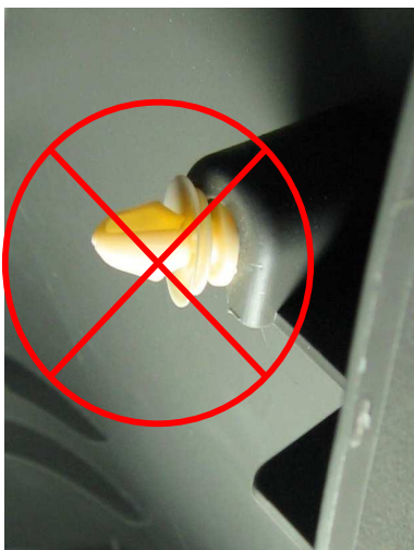
check that the clips on the interior trim are in place.
