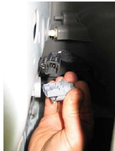
Retrieve the connector from the joint
