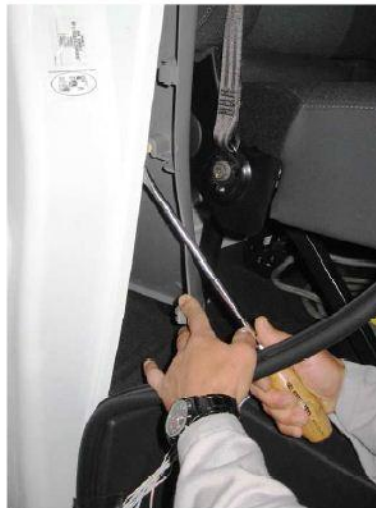
Lever with a flat tool to unhook the lower section of the trim
