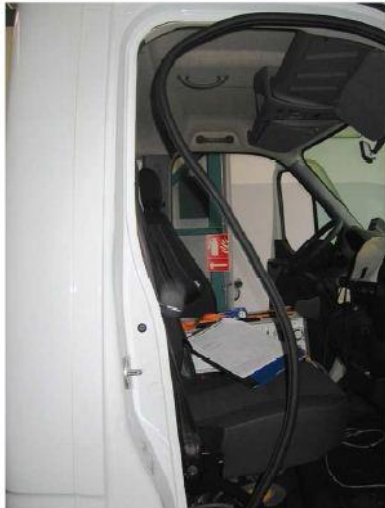
Locally remove the door entry seal on the "B" pillar side.
